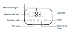
The machine is equipped with six buttons: "power button", "function selection", "increase temperature", "reduce temperature", "time" and "night light", as shown below:
