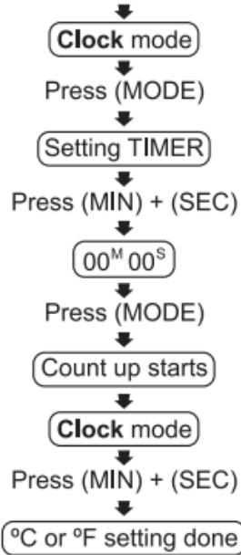
**D Unit temperature (°C / °F) set up**
